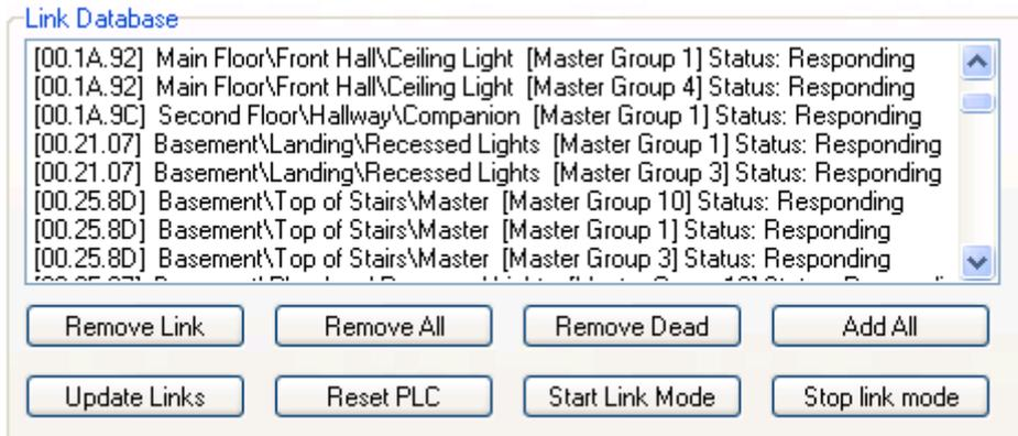
If a device fails to respond to a message, the Link Database shows **No Response** followed by the number of messages the device has failed to respond to in brackets.
